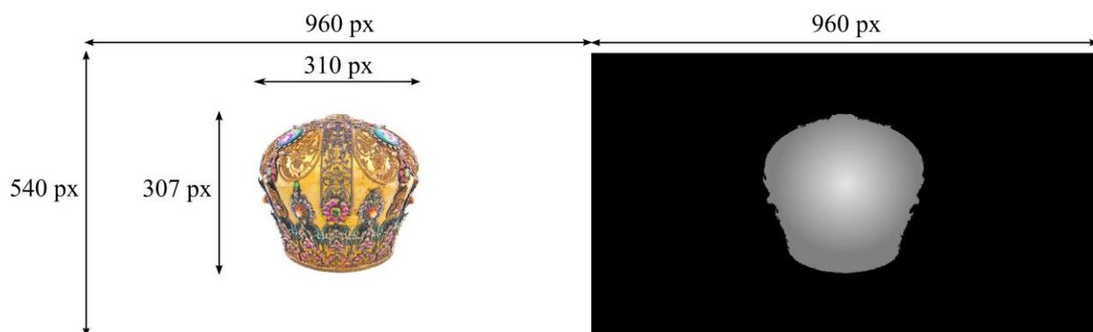
Fig. 6: 3D image (image plus depth) for 42'' autostereoscopic display.
