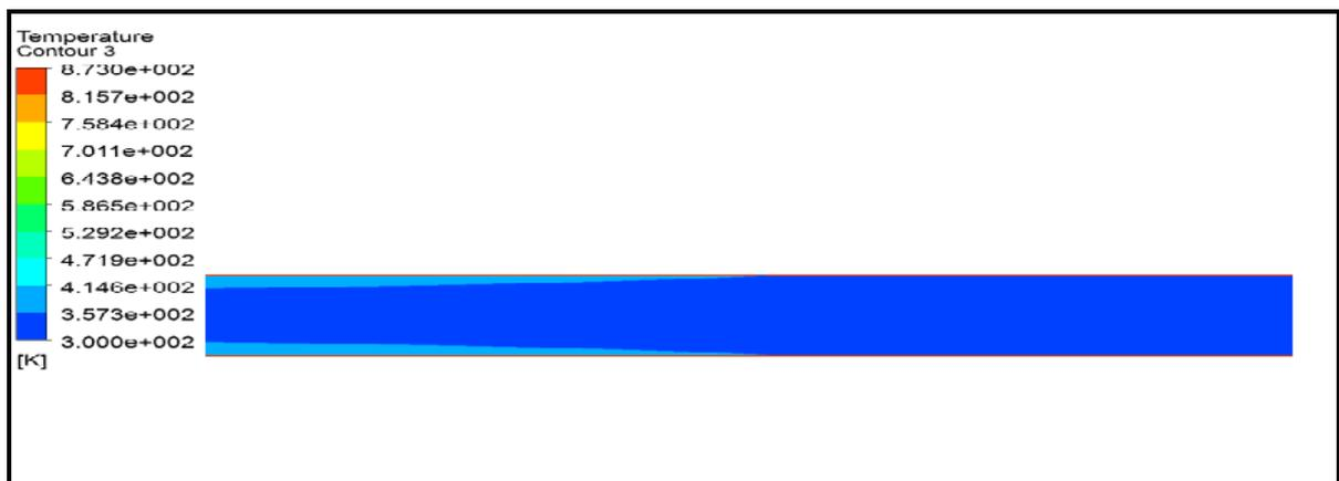
Figure(5) Contour of temperature distribution for smooth duct at surrounding hot air temperature of (873K<sup>o</sup>)
