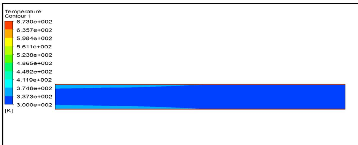
Figure(1) Contour of temperature distribution for smooth duct at surrounding hot air temperature of (673K<sup>o</sup>)
