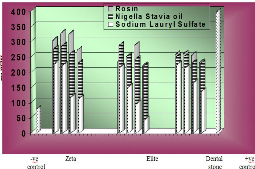
Figure 1. The Effect of Chemical Additives on the Compressive Strength of Dental Stones.
