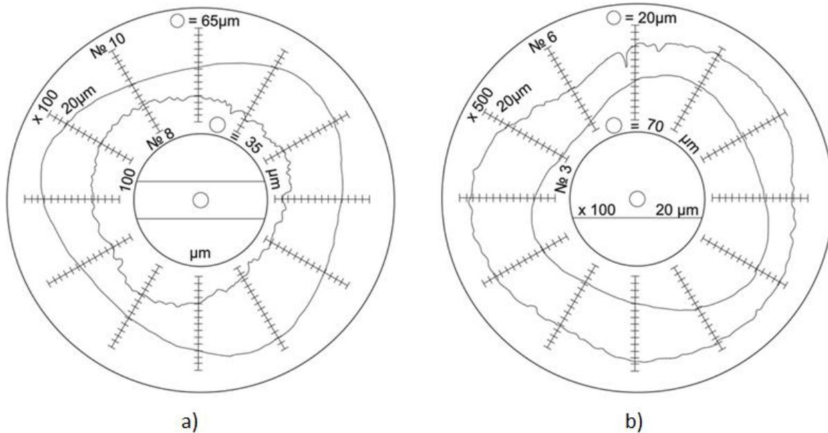
Fig.5. Circlograms obtained by machining holes with prefabricated drill bits.
