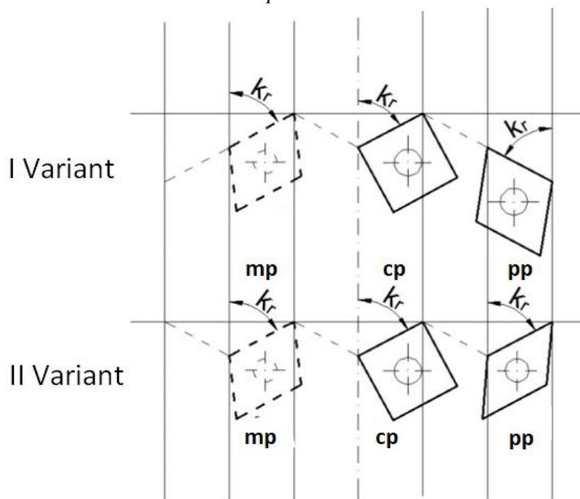
Fig.3. Schemes of cutting inserts placement in deep hole drills. I variant - with sequential cutting insertion of the cutting tips; II variant - simultaneous cutting insertion of the cutting tips (pp - peripheral plate; cp - central plate; mp - middle plate).
