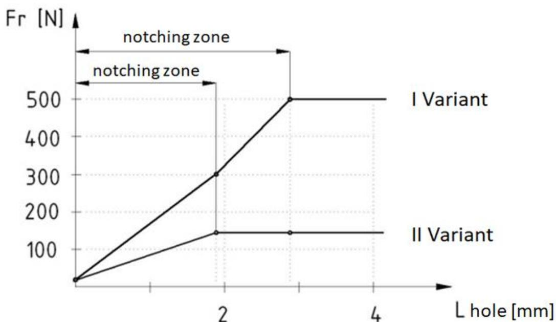
Fig.4. Variation of radial force versus notch length.
