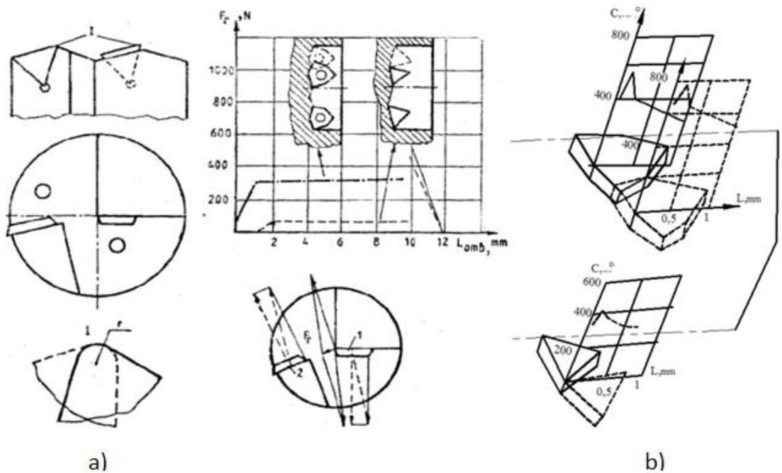
Fig.2. Progressive notching scheme. a) radial force variation; b) thermal loading of notching tips.
