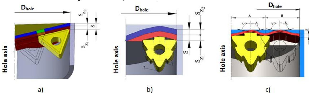
Fig.1. Cutting schemes of the additive in drills with replaceable carbide inserts RCI.
