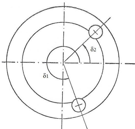
**Fig.6** Arrangement of the guide rollers of an annular drill
