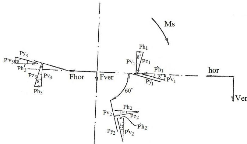
Fig. 4 Loading scheme of annular drill
