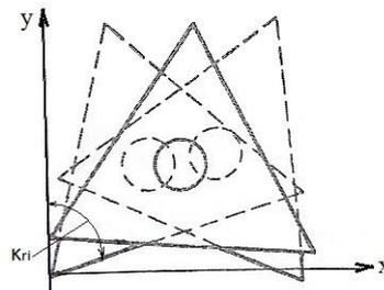
**Fig.3** Scheme of the sequential layout of the cutting inserts
