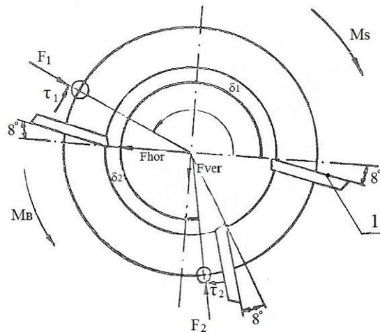
Fig. 5 Scheme for determining the angles  $\delta_1$  and  $\delta_2$  of the position of the guide rollers
