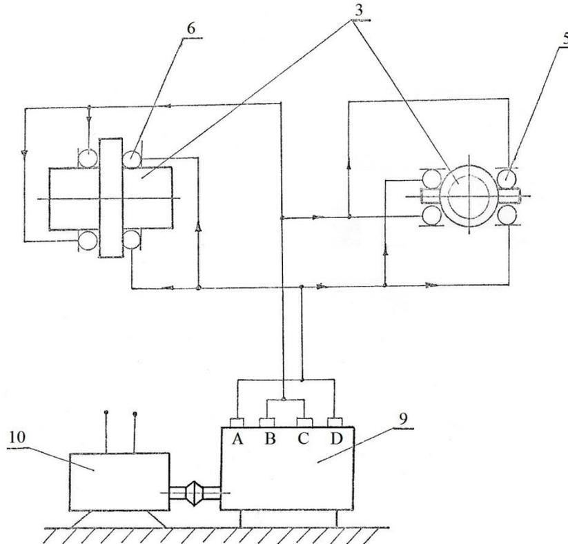
**Fig.4** Hydraulic vibrator connection diagram
