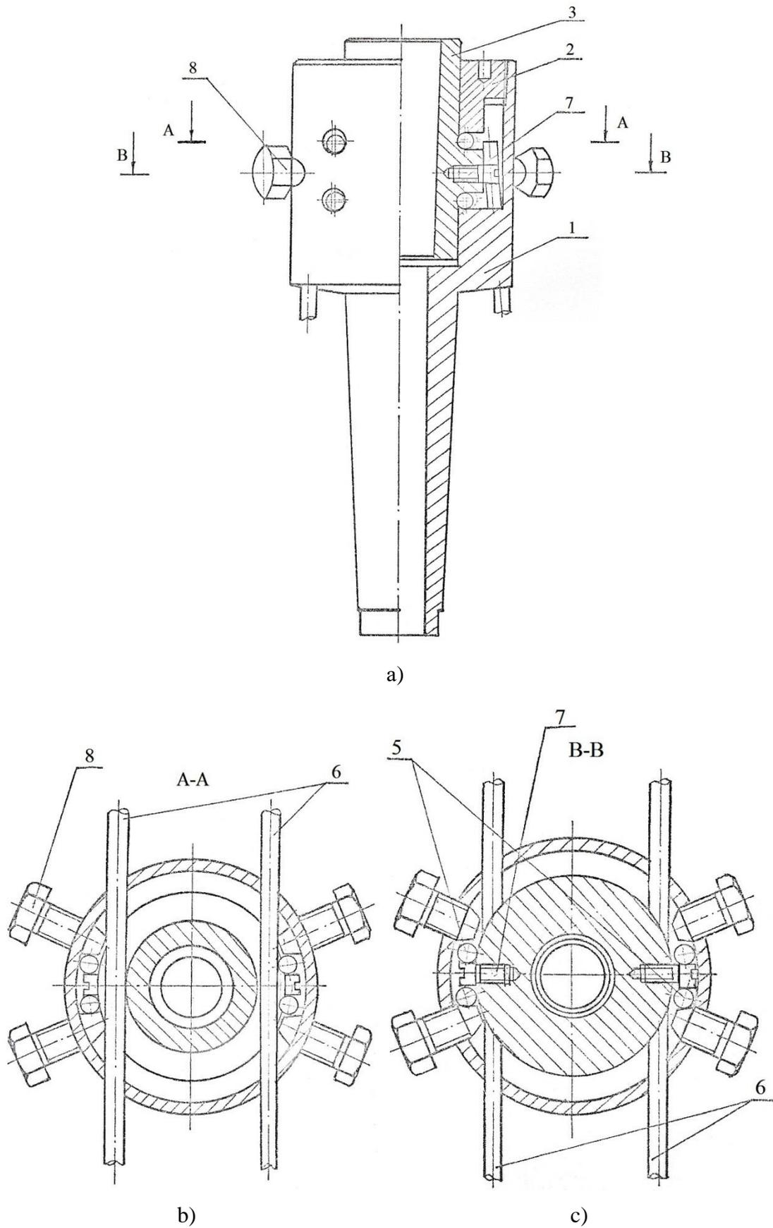
**Fig.3** Design of the vibrator
