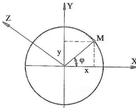
**Fig.2** A scheme showing a point on the cutting edge without vibration
